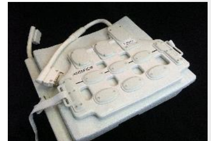
Torso Xenon RF coil Multi element array RF coil for thoracic imaging in MR
