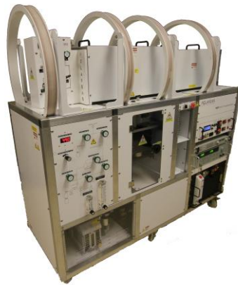
Polariser Uses laser technology, cryogenics, and magnetic fields to excite Xenon spins
